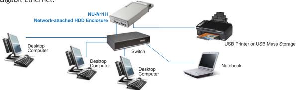
The USB host port can connect to a USB device, such as a extra HDD or card reader to expand storage capacity or a USB printer.
