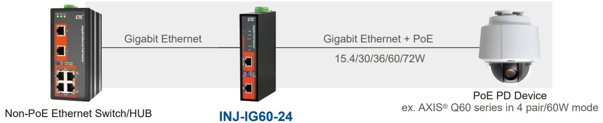
Figure 2 : Very high efficiency boost technology for PoE
