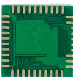
BT10-1 is a multi-protocol RF module using NORDIC SoC nRF51802. This module is ideal for low power wireless sensing device applications such as mobile phone accessories, sports, fitness equipment, consumer electronics, HID, health care, and etc.. The module has been designed to provide ultra-low power, low cost and robust 2.4 GHz communications and compliant with Bluetooth Version 4.2 low energy (BLE, Single Mode) solution.
