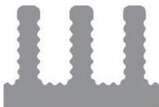
Waved surface heat-sink fins for maximum cooling performance
