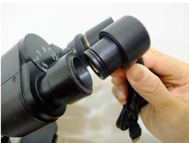
Electronic eyepiece is inserted into the standard
